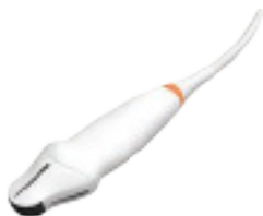
MC9-3TQ 3 - 9 MHz Micro-convex Array Equine hoof, abdomen, cardiac
